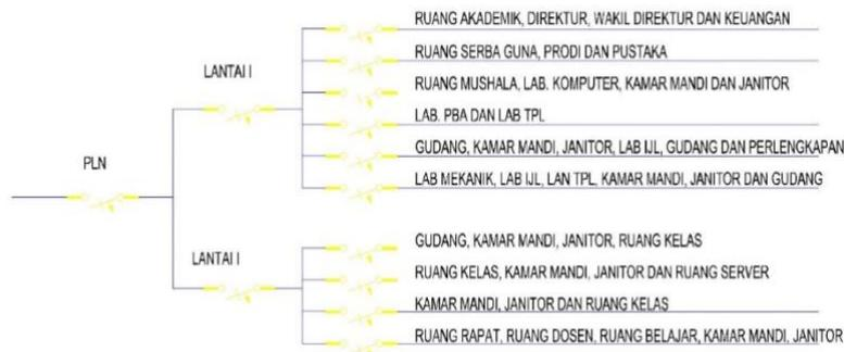
Gambar 4. Single line diagram distribusi daya di AKN aceh barat
